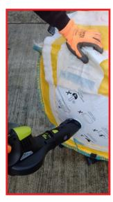
Insert the Inflator through the valve and inflate with the Inflator at maximum.
